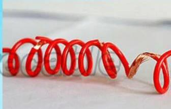
**Inferior** Jacket damaged , reveal conductor
