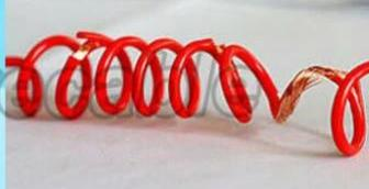
**Inferior** Jacket damaged , reveal conductor
