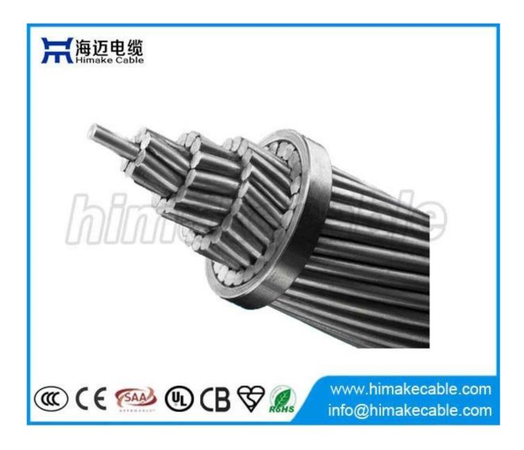
**Conductor structure:** The conductor consists of Aluminum Magnesium-Silicon alloy wires stranded in successive layers in opposite direction and the outer layer is right hand direction Z, Natural grease may be applied between the layers of AAAC except the outer layer.
