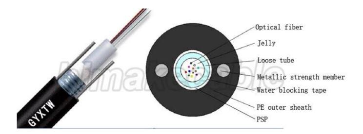
2~24 fibers, jelly filled, fiber contained central loose tube copolymer coated steel tape, two parallel steel wires 1.2mm
