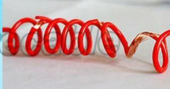
**Inferior** Jacket damaged , reveal conductor
