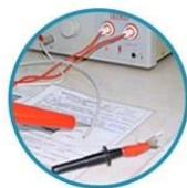
Insulation resistance test
