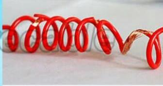
**Inferior** Jacket damaged , reveal conductor
