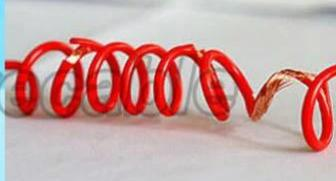
**Inferior** Jacket damaged , reveal conductor
