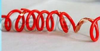
**Inferior** Jacket damaged , reveal conductor
