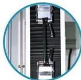
Tensile strength test
