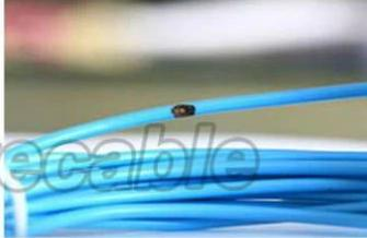
**Inferior** Jacket damaged , reveal conductor
