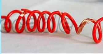
**Inferior** Jacket damaged , reveal conductor
