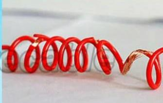
**Inferior** Jacket damaged , reveal conductor
