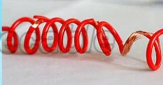
**Inferior** Jacket damaged , reveal conductor
