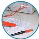
Insulation resistance test
