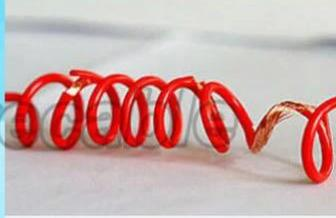
**Inferior** Jacket damaged , reveal conductor
