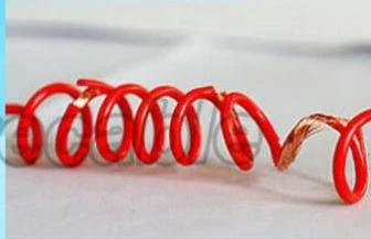
**Inferior** Jacket damaged , reveal conductor
